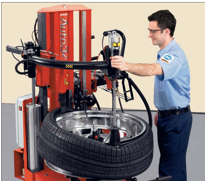
Bead press arm during mounting, places tire in drop-center for mounting.
