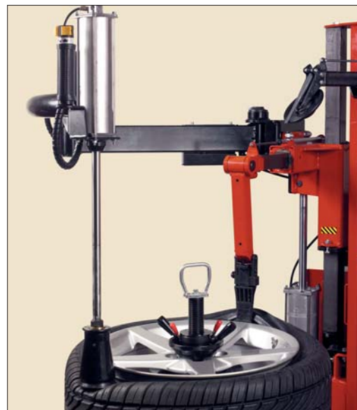
Bead press arm eases de-mounting of a standard tire. Used to press opposite side of tire into drop-center.
